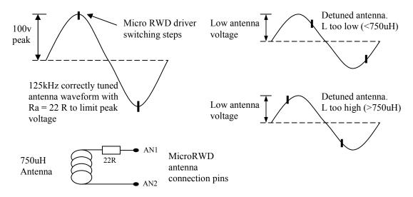
6) For optimum performance the antenna Q should not exceed 20 and to achieve reliable tuning at 125kHz the antenna inductance should be around 750uH. Higher Q and inductance values will still function but with a reduced range and performance.
