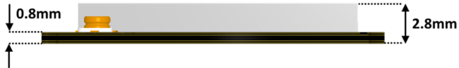
Figure 4-1. Pepper C1 FCC module dimension
