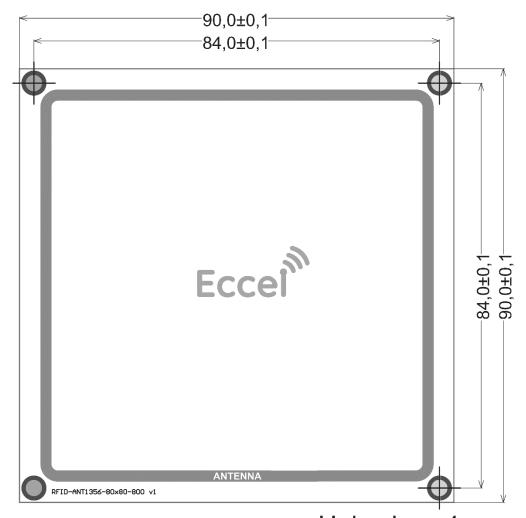
Hole size x4 Ø 3.4 mm Outer diameter Ø 5.0 mm
