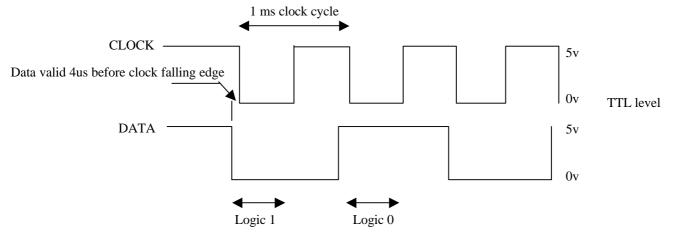
Data stable before clock falling edge and while clock low
