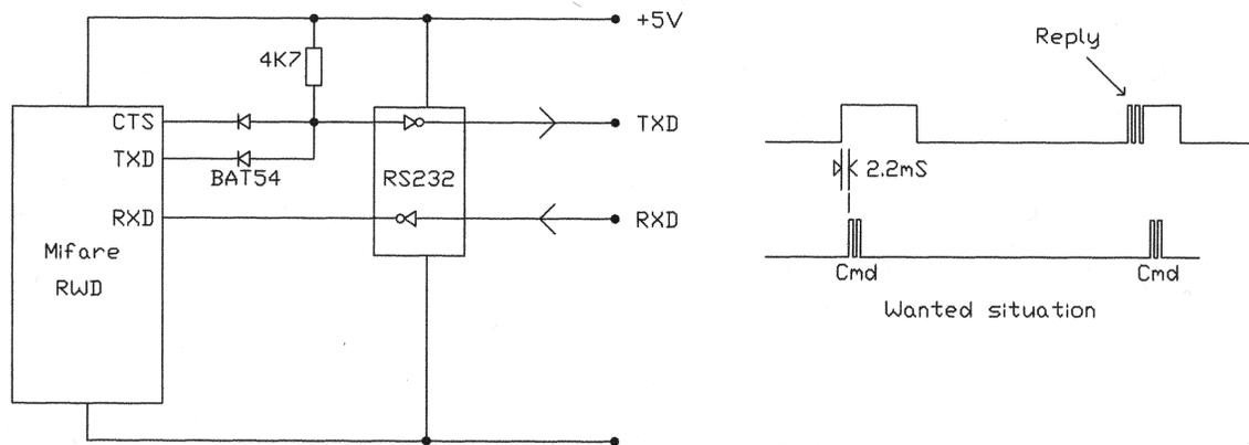
Note the inversion of signals through the RS232 level converter device (such as MAX202)
