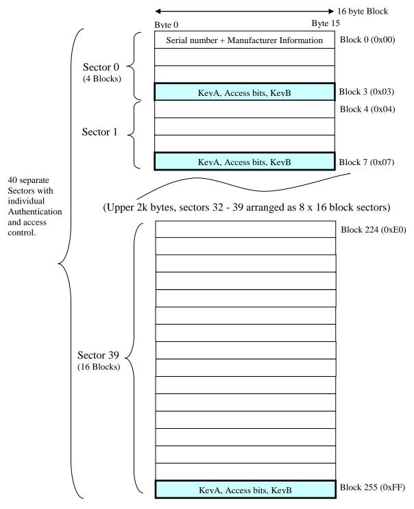
The lower 2048 bytes of the 4k card (sectors 0-31) are organised in the same way as the 1k card. However the upper 2048 bytes are organised as eight large sectors of 16 blocks each (sectors 32-39). Taking into account the Serial Number/Manufacturers Block and the Sector Trailer Blocks then there are 3440 bytes of free memory for user storage.
