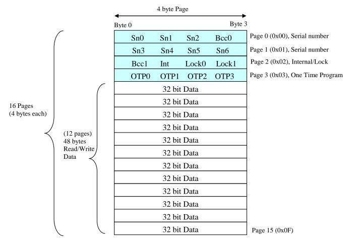
**Note:** Ultralight card has 7 byte serial number (+ 2 check bytes)
